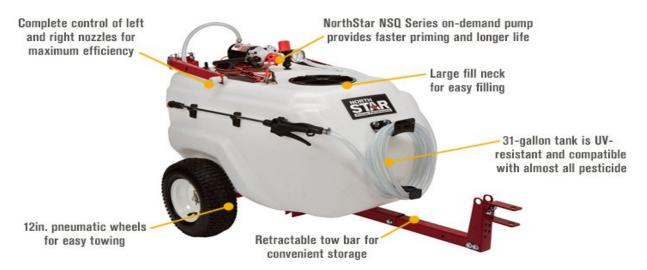
12V 2.2 GPM open flow NorthStar NSQ Series on-demand pump provides faster priming and longer life; 70 PSI max.
